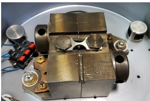
Fig. 1. Installation for carrying out experiments on thermal fatigue.
