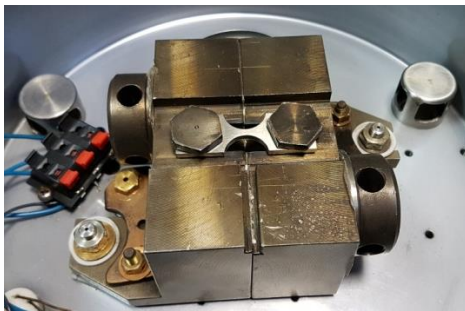
Fig. 1. Setup for thermal fatigue experimental investigations.
